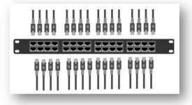
A PoE Midspan (injector) adds power but does not manage the data. Each "Poe out" port has its own "data in" port
