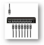
A PoE Switch adds power and routes data between devices. One data connection in, multiple ports of power and data out.
